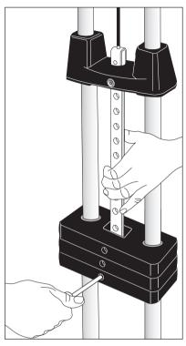
Hold the stem in place by inserting the Weight Pin (through a weight) near the base of the Selector Stem.
